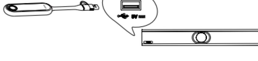
1. Connect the WPP30 to the USB-A port on the endpoint.
